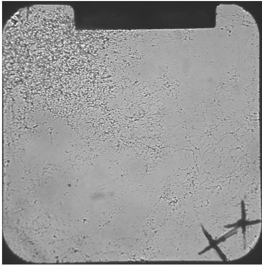
Figure 7. In their optical cryostat, Sasaki et al [70, 63] could grow solid helium samples at constant volume in a time of order one hour as usually done in TO experiments. This photograph shows that the sample is polycrystalline. The window is 11 mm wide. The grain boundaries are revealed by lowering the pressure to the melting pressure P_m = 25.3 bar so that the contacts of grain boundaries with the cell windows are invaded by liquid helium (see section 4.2).
